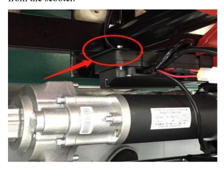
Step 5: Using cross screwdriver or straight screwdriver to unscrew the four screws of the motor controller, and you will see those wire connections here.
