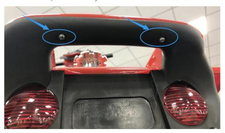
Step 3: Open the rear cover as the below and plug off the white connectors. It is the connection of motor controller and scooter (you must reconnect the white plug after step 7)
