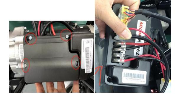
Step 6: Plug off the connectors as below and then check the pins arrowed in place.
