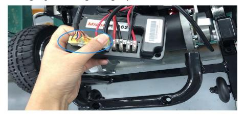
Step 8: Now you shall reconnect the white plug of the motor controller I mentioned above, and turn on the scooter to check it works or not.
