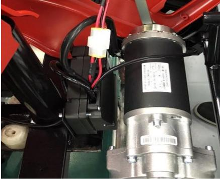
Step 4: Take off the one bolt on the controller by M3 hex wrench from the scooter.
