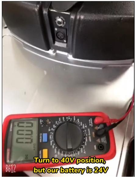
3. Insert the detection head into the battery case. Please note the positive and negative poles. Red line is for the positive, and the black is negative.
