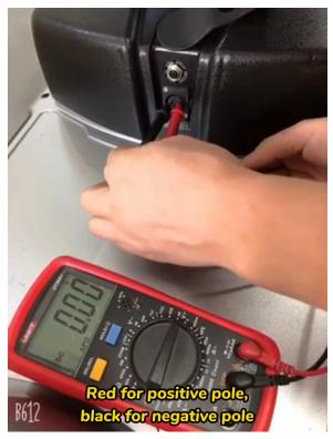
4. For a normal battery, the voltage will around 27V under full charging. If the voltage is lower than 24V after full charging. The battery can not hold the battery and shall be replaced.
