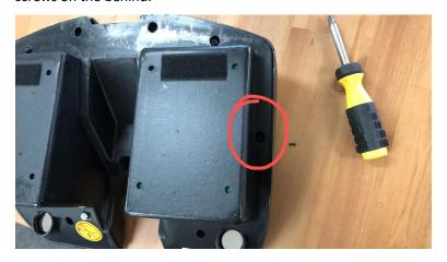
5. Finally, be careful with the front two screws. You must tighten them with your hands and then lock them, otherwise the threads may be damaged by mismatching.
