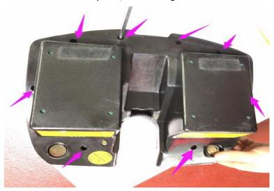
2. Find the screw of the handle, and loosen the screws, take out the handle, exchange a new one on it.
